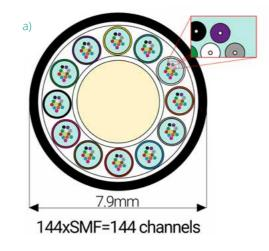
Fig. 1. a) Fiber optic cable with SMFs; b) Fiber optic cable with InPhoTech's MCF.
