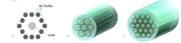
Fig. 4. a) MCF's basic cell; b) 7-core fiber design; c) 19-core fiber design
