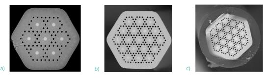
Fig. 7. Microscope images of the cross-section of a) 7-core fiber b) 19-core fiber c) 19-core fiber with coating.
