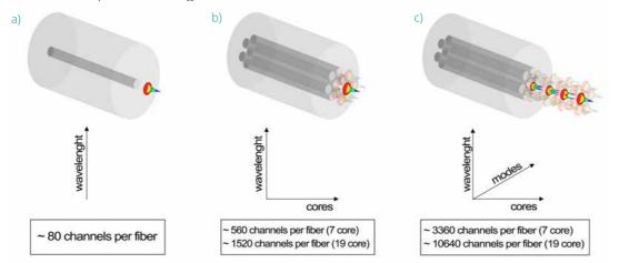
Fig. 3. From today to the future with InPhoTech's MCF. a) SMF + WDM; b) MCF + WDM; c) MCF + WDM + MDM
