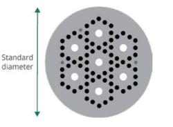
Fig. 5. InPhoTech's MCF structure with its characteristic elements.
